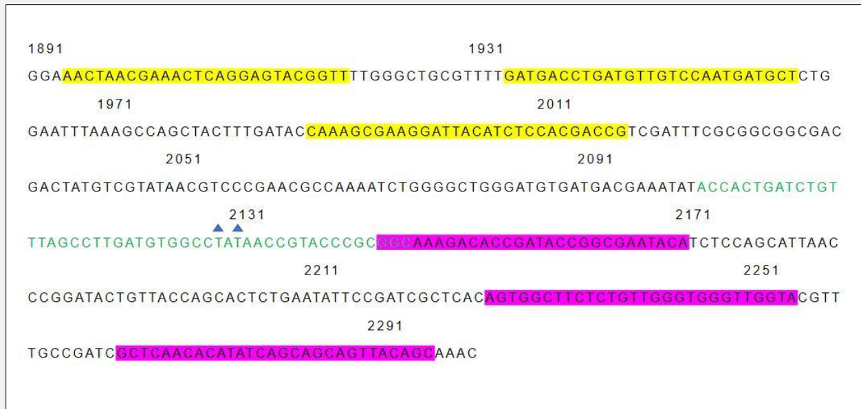
Figure 1. Position of primers and probe on chuA gene.
